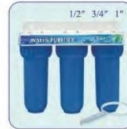
UMK-BR10B5 Triple filtration PP+GAC+CTO Inlet pressure: 8-125 PSI. 0.6-8.8 kg/cm 2 With steel bracket, wrench.
