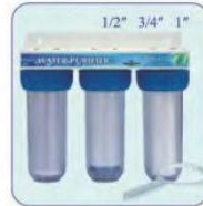
UMK-BR10B4 Triple filtration PP+GAC+CTO Inlet pressure: 8-125 PSI. 0.6-8.8 kg/cm 2 With steel bracket, wrench.
